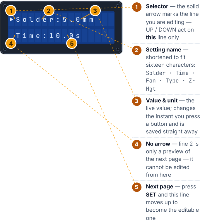
Figure 02.1 — The settings display. Sixteen characters by two lines, exactly as the machine draws it.
