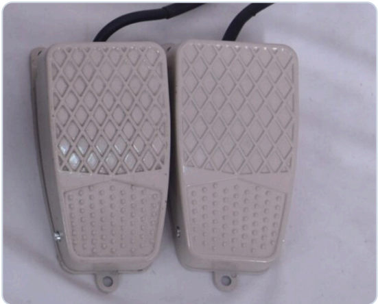
Figure 01.2 — The two pedals. Mark them; they are identical outside and do very different things (§06).
